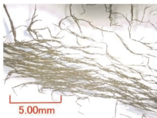
Figure 2. Photograph of magnetic clusters of MCF (Cu at 3 g, Ni at 3 g, MF at 4 g).
